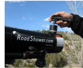
Joel pressurizes Road Shower with a CO 2 pump.
